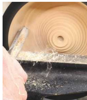
▲ Pic.10 A series of steps helps you gauge the position of the tool throughout the process. The bulk of timber in the centre will help to give some stability to the bowl
